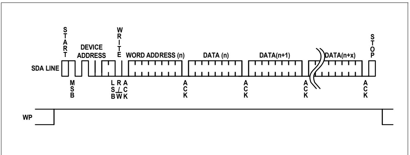
**Figure 11. Non-Write-Protect Condition**
