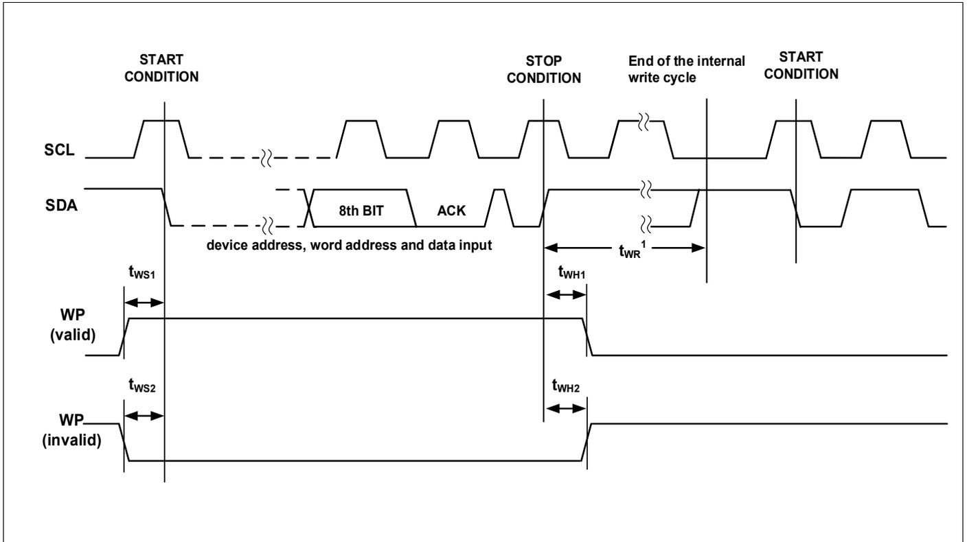
Note: 1. The write cycle time  $t_{WR}$  is the time from a valid stop condition of a write sequence to the end of the internal clear/write cycle.
